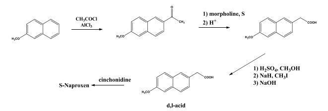
Scheme (5): First large-scale naproxen process (500 kg)
