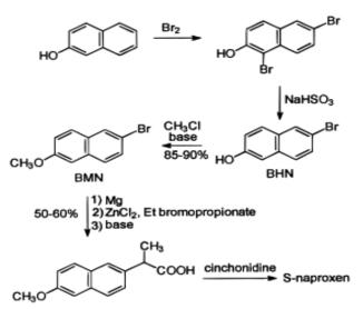
Scheme (6): First large-scale manufacturing process, 1972-1975
