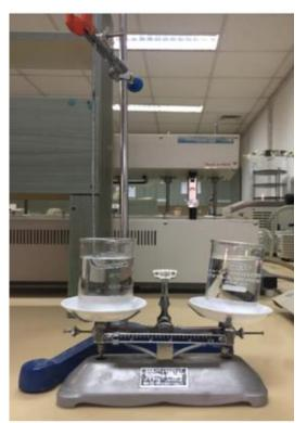
Figure (1): Double pan balance and the wire probe used for raft strength measurement (modified method).
