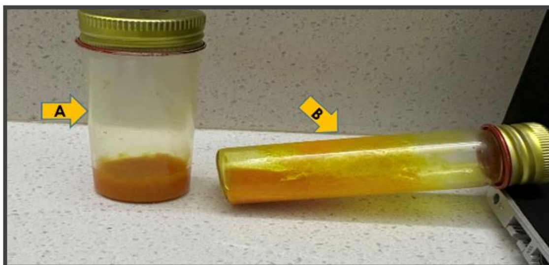
Figure 2: Thermal behavior of the organogels (A) Semi-solid state of the organogel at room temperature and (B) sol state of the organogel at 39 °C and above temperature.
