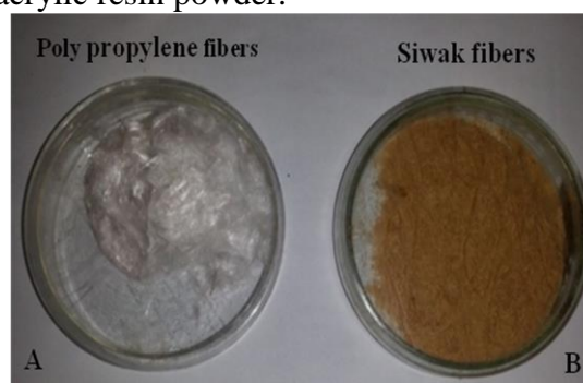
Fig.1: Silanized. A, poly propylene fibers; B, siwak fibers.
