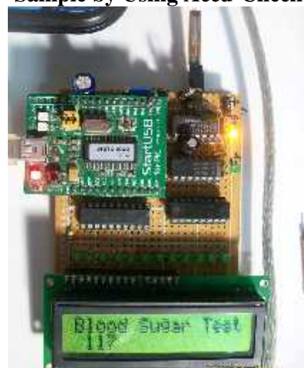
Figure-14: The Result for the First Blood Sample by Using the Prototype Circuit
