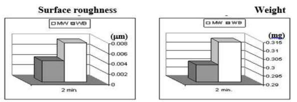
Figure-8: Histogram showing the effect of conventional dental lathe (as control group) on the mean surface roughness and the mean weight were cured by two methods.
