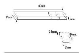
Figure-1: Specimen dimension and location of surface cuts.
