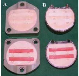
Figure-2: A- Wax plate mold in the fiber reinforce plastic flask. B- Wax plate mold in the dental flask.
