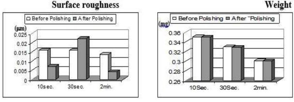
Figure-10: Histogram showing the effect of the polishing on the mean surface roughness and the mean weight in the WB method (before and after polishing).
