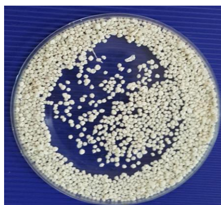
Figure 1. An image of uncoated calcium alginate beads loaded with mefenamic acid (F3).
