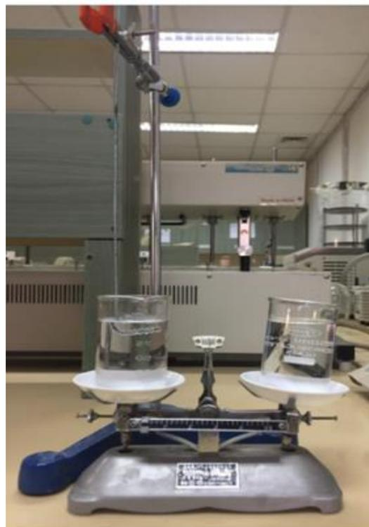
**Figure (1): Double pan balance and the wire probe used for raft strength measurement (modified method).**
